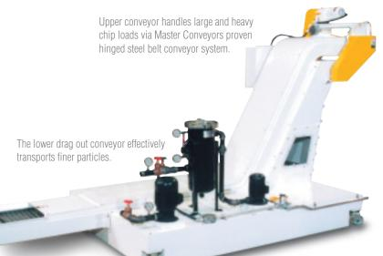
Liquid tight viewing window allows for visual inspection of filter system.
